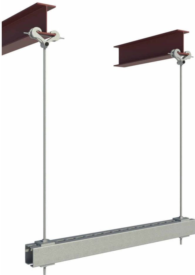
TRAPEZE CONNECTION DETAIL (TYP)
